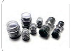
The Push-Fit Coupler makes coupling of MicroDuct fast and easy. Simply push the MicroDucts into the center of the Push-Fit Coupler. No tools are required. Push-Fit Couplers can be connected and disconnected for maintenance and still maintain the high performance requirements for Blown-In fibre systems.
