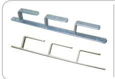
The Type F Bracket is a robust support manufactured from 5mm thick mild steel and has a galvanised finish. It has four 8mm holes through which it is bolted into a wall.
