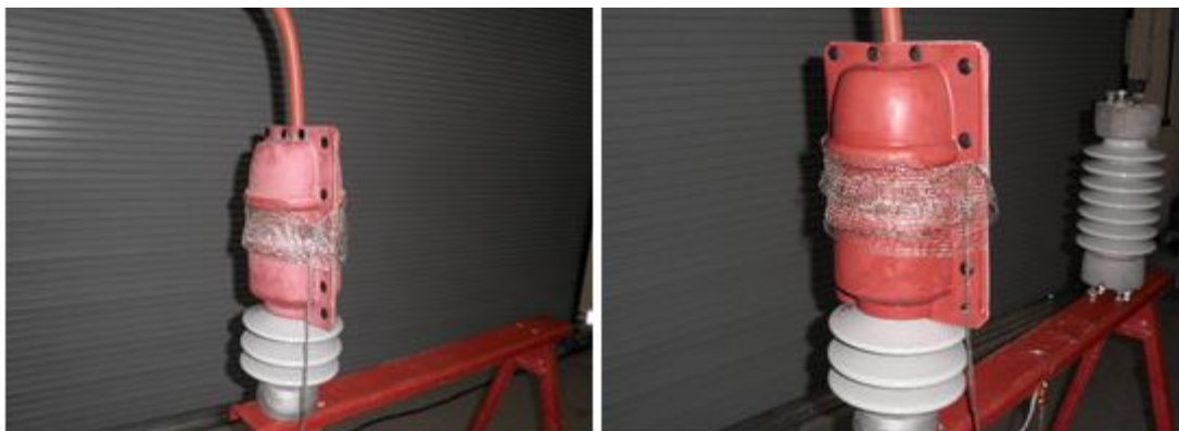
Figure 10 AC Withstand Test Set up showing the product with 12 years in-field service (left), which is heavily contaminated with residue on the inside and outside and new unexposed cover (right), the steel mesh represents a ground plane
