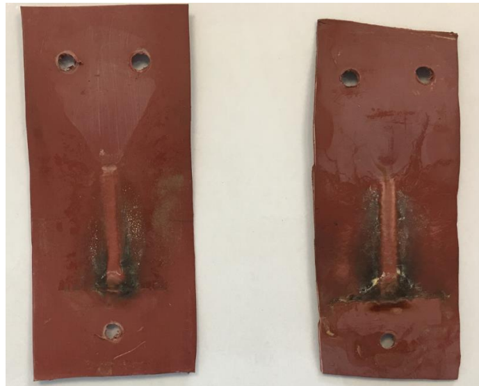
Figure 8 Tracking and Erosion Test Samples Post 6 hours IEC 4.5kV Constant Test: (left) BCIC Control Product; (right) BCIC In-Field Service Product
