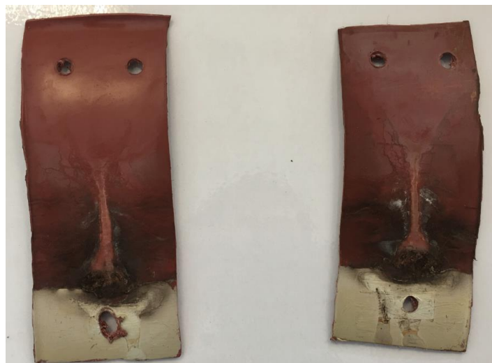
Figure 7 Tracking and Erosion Test Samples Post 5 hours ASTM 2.5kV Step Test: (left) BCIC Control Product; (right) BCIC In-Field Service Product
